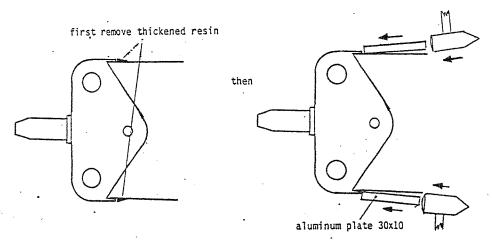
Next sandblast the fitting(Using only approved material) and apply a fresh corrosion pretection. Then carefully smooth the spar stub (using a 400 grid sand paper), apply a thin coat of resin, push fittig fully home and install hollow rivets. The step between fitting and stub and between connecting glass layers should be filled uo using thickened resin.
